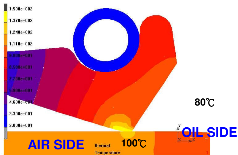
<Figure 5.1> The seal lip temperature will raise over 20°C in normal operation
